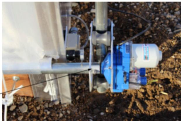
Align roll-bar, roll-bar adapter, and motor shaft bolt holes. Then, fasten securely with the bolt and nut.
