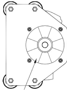
Roll-bar goes thru large hole and bolts to output shaft
