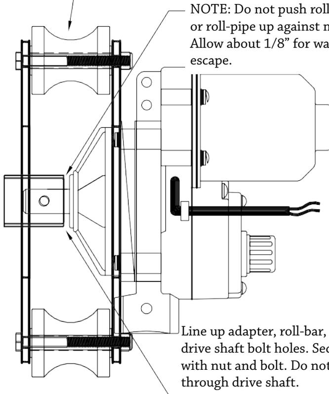
NOTE: Do not push roll-bar or roll-pipe up against motor. Allow about 1/8" for water to escape.
